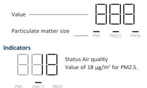
The 70-models have a dynamic screen control that shows additional values and statuses for different categories, and have additional indications to show active functions. Press the left or right arrow to switch between the different categories.
