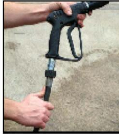
Attach trigger to high pressure hose.
