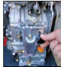
Push throttle into 'start' position and tighten knob.
