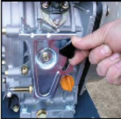
To switch off unscrew knob and move throttle to the 'stop' position..
