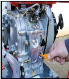
Check engine oil and replenish as required.
