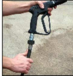
Attach trigger to high pressure hose.
