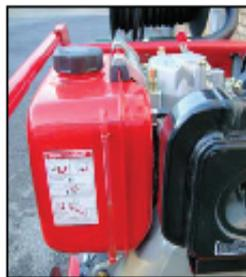
Check diesel using sight measure and replenish as required.
