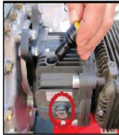
Check gearbox oil using dipstick or sight glass - replenish as required.
