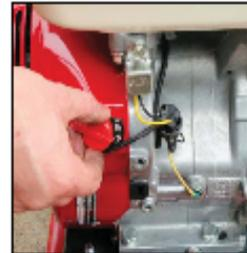
Turn engine switch to 'on' position.
