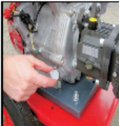
Check engine oil and replenish as required.
